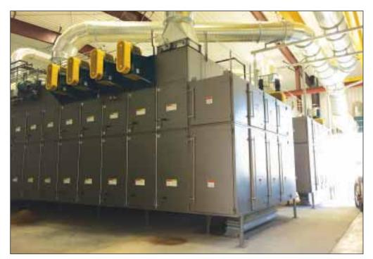
Two Bühler Aeroglide dryers replace conventional pellet coolers at the Ainsworth mill. They are designed to increase range cube shelf life by removing all water activity. Photo courtesy of EBM Construction Inc.
